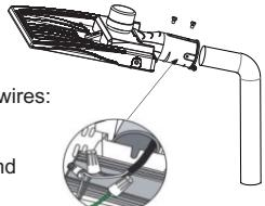
4. Install slipfitter onto lamp pole
