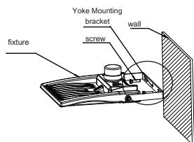
2. Mount Yoke Mounting bracket onto the wall
