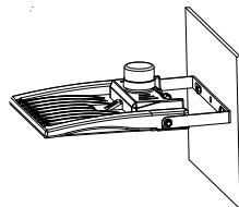
3. Put the cord through the Yoke Mounting Bracket and connect wires
