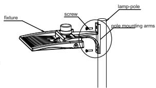
3. Connect the wires to the wires that are coming from the lamp pole
