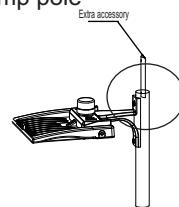
If fixture is installed onto a square lamp pole, install the extra accessory before Step 4 above, the rest of instruction are the same
